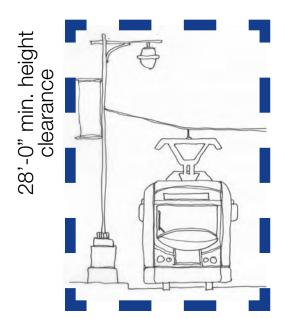
Estimated height clearance for streetcar/trolley. An easement should be established throughout the proposed route to maintain this easement for future trolley.
