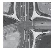
Main and College intersection is currently serving volumes over its built capacity. Due to the pedestrian underpasses, improvements to the intersection will need to be innovative.
