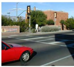
High-intensity Activated crossWalk (HAWK) signal is dark unless activated by a pedestrian. Photo courtesy of Nelson | Nygaard.
