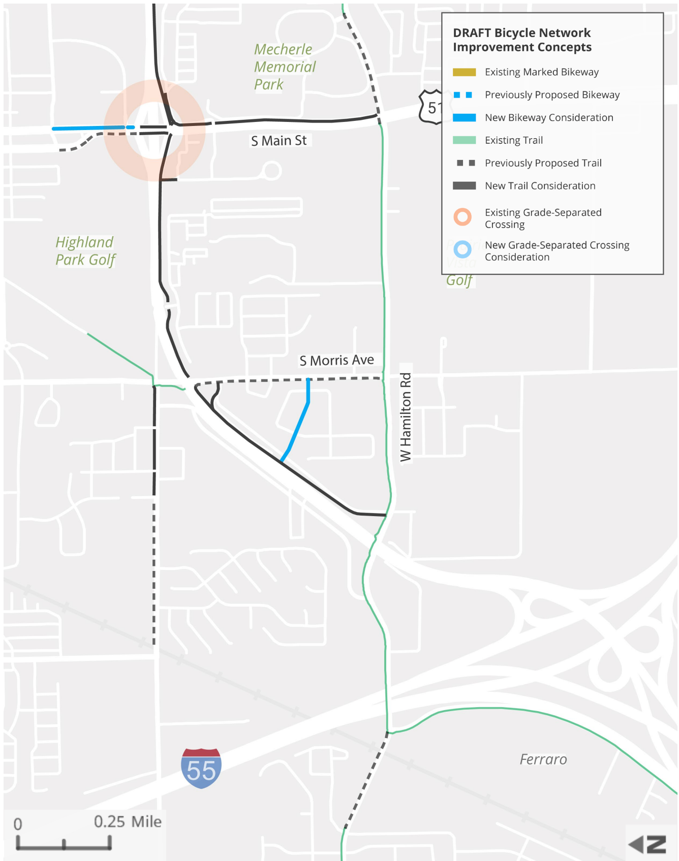
Figure 34: Bicycle Network Improvements - Main Street to I-55
