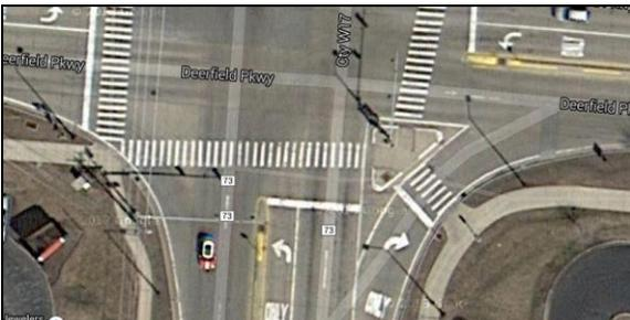
Figure 2.4. Top: Bringing sidepath crossings closer to the parallel road. Bottom: Right-turn corner island and high-visibility continental crosswalks
