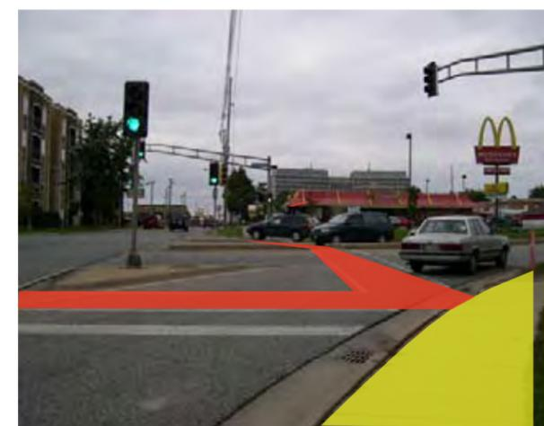
6 Red Pathways. Crosswalks are necessary for the flow of pedestrian traffic, however, they should be designed in such a way as to minimize their length.
