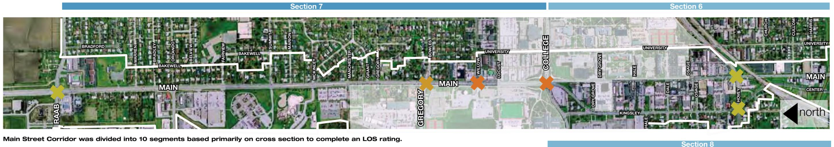
Main Street Corridor was divided into 10 segments based primarily on cross section to complete an LOS rating.
